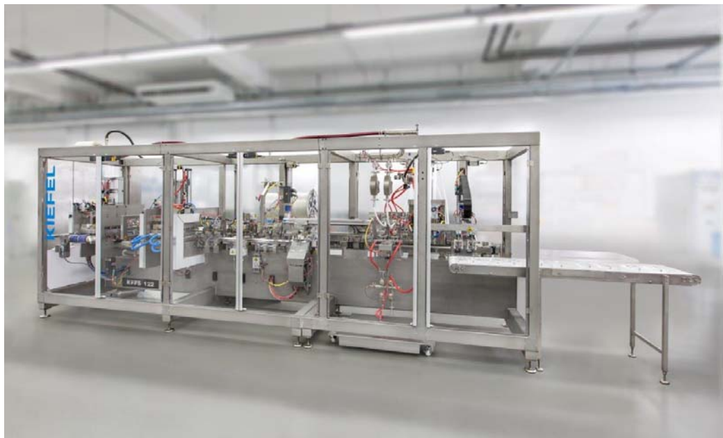
Image: Thermal-contact Form-Fill-Seal-Machine KFFS 122 for the Production of Infusion Bags
